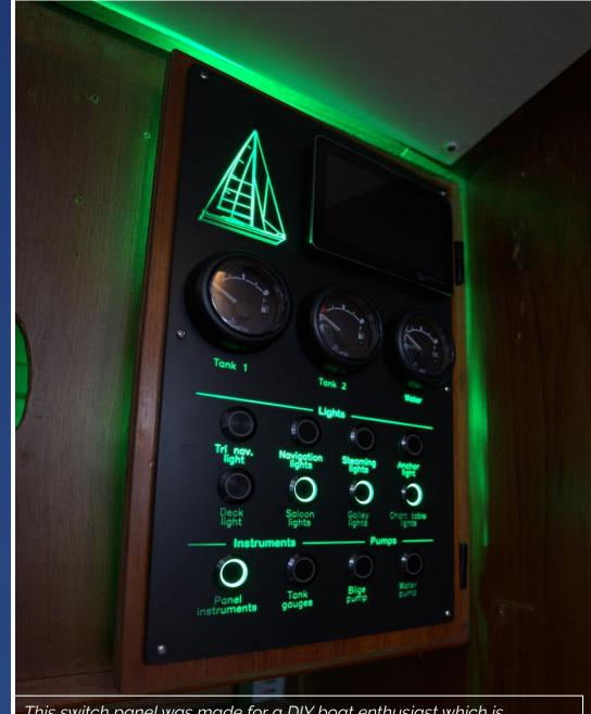
This switch panel was made for a DIY boat enthusiast which is completely rebuilding his boat. With all the new electronics installed, a custom made distribution panel made much sense!
